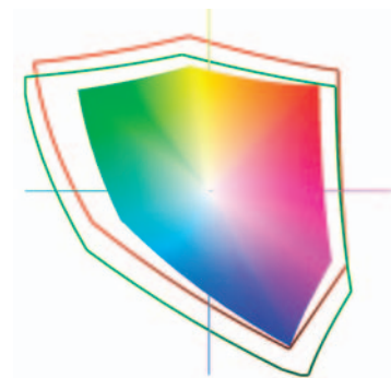
This graph depicts the color range of a Sony Artisan monitor against Adobe RGB (green) and the Eizo ColorEdge CG220 (red). Notice that the CG220 has almost the same shape and color gamut of the Adobe RGB color space.
